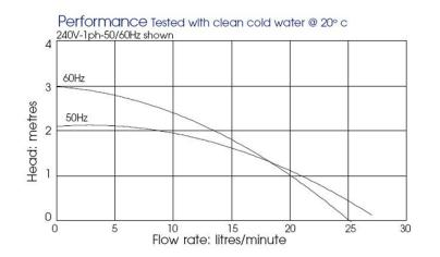
NOTE: These magnetically coupled pumps are designed for use with clean fluids.
