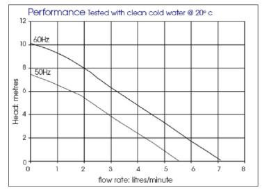
NOTE: These magnetically coupled pumps are designed for use with clean fluids.
