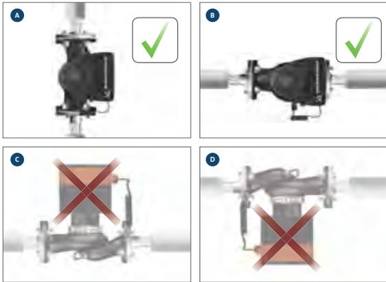
Fig. 53 Installation positions
