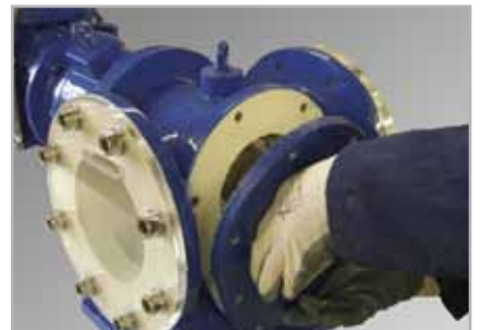
6. Inspect/replace cutters, spacers and shafts
