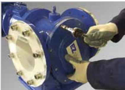
4. Loosen and remove shaft lock nuts
