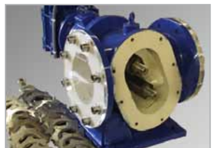
6. Inspect/replace cutters, spacers and shafts
