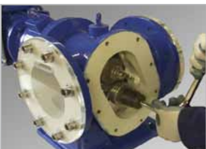
4. Loosen and remove shaft lock nuts
