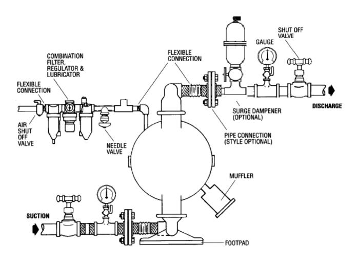
**NOTE:** In the event of a power failure, the shut off valve should be closed, if the restarting of the pump is not desirable once power is regained.
