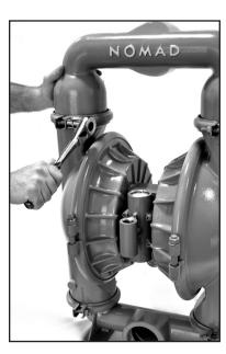
**Step 2:** Utilizing the 11/16" socket wrench, remove the two small clamp bands that fasten the discharge manifold to the liquid chambers.
