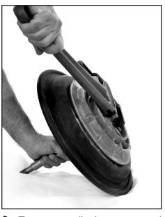
**Step 10:** To remove diaphragm assembly from shaft, secure shaft with soft jaws. Using an adjustable wrench, remove diaphragm assembly from shaft.
