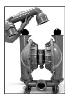
**Step 3:** Remove the discharge manifold to expose the valve balls and seats. Inspect the ball cage area of the manifold for excessive wear or damage. Remove the discharge valve balls, seats and o-rings from the discharge manifold and inspect for nicks, gouges, chemical attack or abrasive wear.
