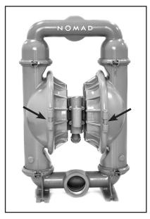
**Step 1:** Before starting disassembly, mark a line from each liquid chamber to its corresponding air chamber. This line will assist in proper alignment during reassembly.
