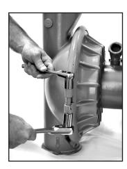
**Step 6:** With 3/4" socket and 3/4" box wrench, remove one set of large clamp bands that attach liquid chamber to center section assembly.
