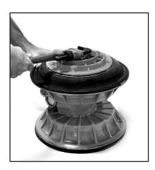
**Step 8:** Using an adjustable wrench, or by rotating the diaphragm by hand, remove the diaphragm assembly.
