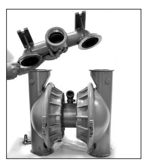
**Step 5:** Lift the intake manifold away to expose the valve balls and seats. Inspect intake valve ball cage for excessive wear or damage. Remove the intake valve balls, seats and o-rings from the discharge manifold and inspect for nicks, gouges, chemical attack or abrasive wear.
