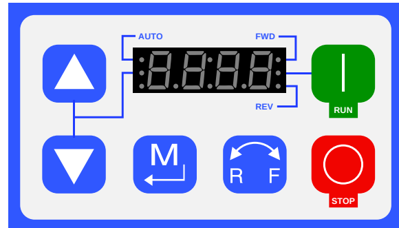
Figure 7 VFD Control Panel
